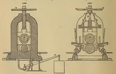
When a slab has entered and passed once through the rolls, the engines are reversed, and the water-valve being opened the ram V rises and hauls in the chain, driving the chain-barrel and causing the tightening-down screws U U to descend and lower both ends of the top roll simultaneously to the required extent. This process is repeated after each passage of the slab through
